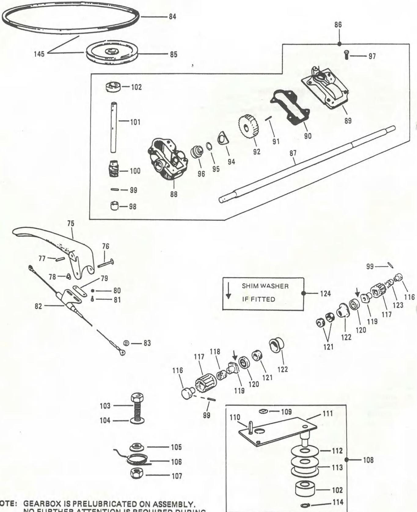
**NOTE:** GEARBOX IS PRELUBRICATED ON ASSEMBLY. NO FURTHER ATTENTION IS REQUIRED DURING ITS WORKING LIFE. AFTER MAJOR SERVICE REPACK WITH NULON GRADE L90 LUBRICANT (147).
